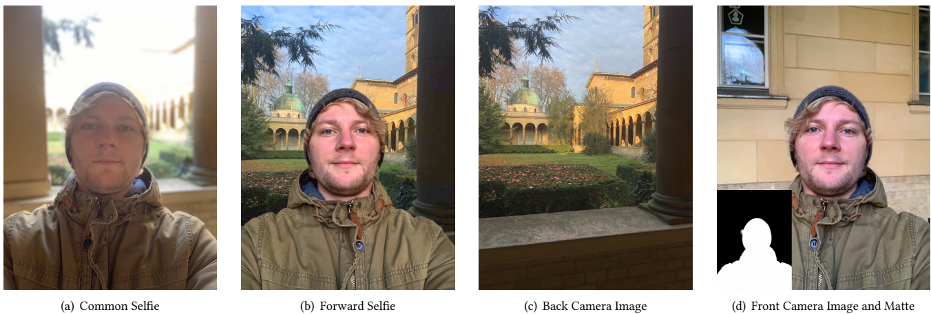
Figure 1: Comparison of a common selfie captured using the front camera (a) and a forward selfie obtained by our mobile application (b). The forward selfie is obtained by blending the back camera image (c) with the simultaneously acquired front camera image using a person-specific matte (d) that is computed during capturing.
