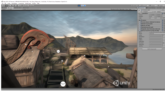
Figure 5: Screenshot of the scene post-processing case study implementation as image effect in the Unity. A Kuwahara filter is applied as last filter to the scene similar to other build-in effects such as Bloom or Antialiasing. The parameters are customized according to the lighting and atmosphere of the scene.
