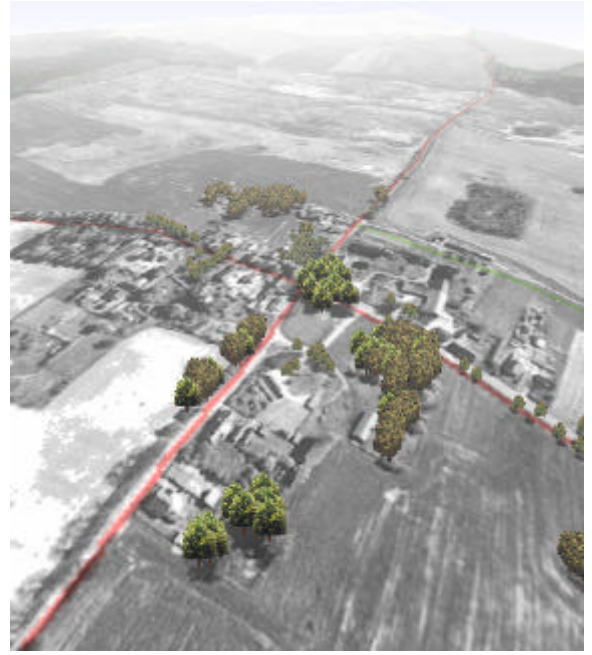
Figure 17. Real-time terrain rendering based on VRS. Lens flares and hazy sun (left) are modeled as OpenGL-specific shapes. Multitexturing attributes are used to display multiple layers of terrain data such as a satellite texture and a road-network texture (right).
