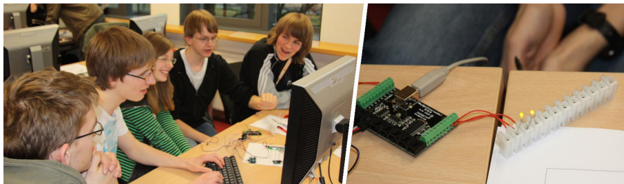
Figure 1: Pupils controlling an LED using Squeak and the Phidget InterfaceKit
