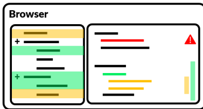
Figure 6. Schematic code browser and editor with color indicators for two active concepts and a warning when names from unrelated concepts have been introduced.
