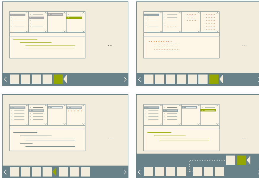
Fig. 4: (From top left to top right) A programmer modifies source code which implicitly creates items in the version bar. The programmer decides to withdraw several changes by going back to a previous version (bottom left), and continues working and creating new changes, which will appear on an new implicitly created branch (bottom right).
