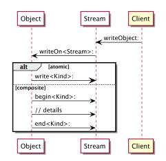
**Figure 9.** Sequence diagram for one cycle of the object/PWS interaction
