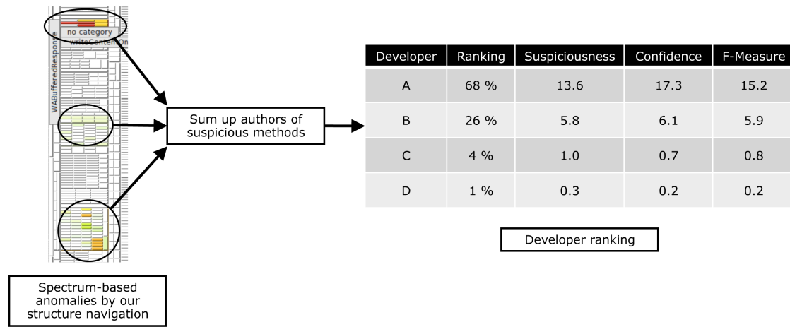
Figure 4.6.: Our developer ranking classifies (anonymized) experts. After analyzing the authors of spectrum-based anomalies, a ranked list presents possible experts that understand failure causes best.
