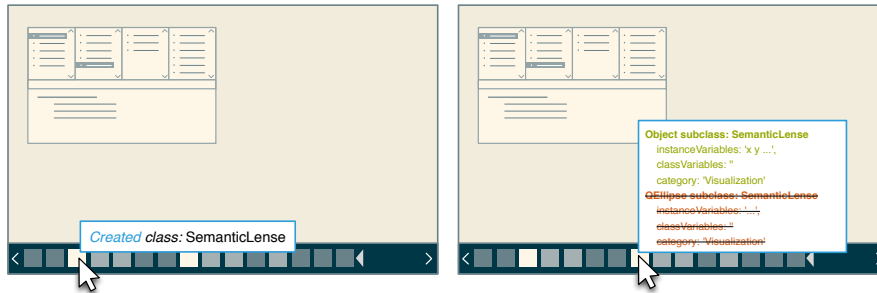
Fig. 3. Hovering shows which source code element has been changed (left). In addition, holding shift shows the total difference to the previous version (right).
