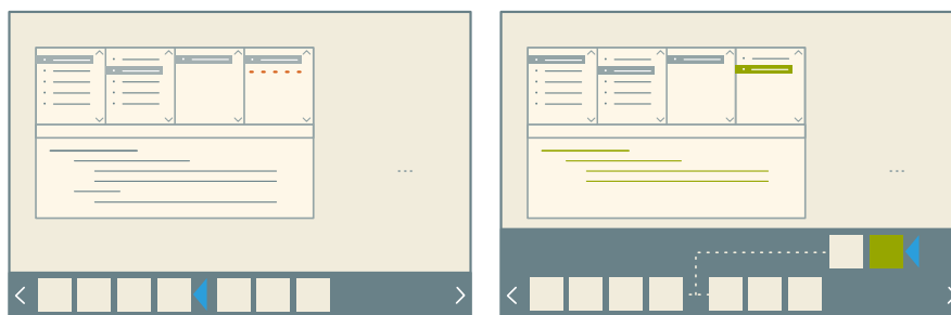
Fig. 2. The (blue) triangle marks the current position in the history - the version that is currently active. When a programmer goes back to a previous version (left), and then continues working, the new changes will appear on a new branch that is implicitly created (right).
